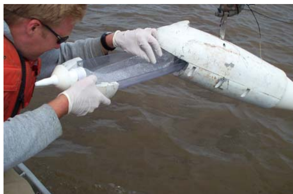
Fig. 2. D-96 depth-integrating sampler.
