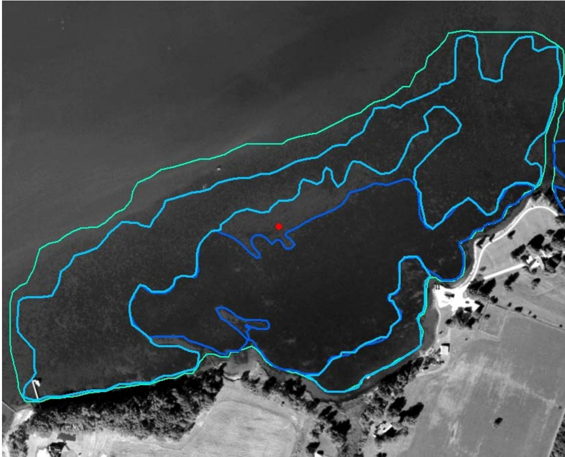
Figure 5. Example of a R. maritima bed that has been digitized according to density. Dense areas are outlined by the dark blue line and moderate areas are outlined by the light blue line (remaining area is considered sparse). The light green line is the bed boundary; red dot is the transplant. Areas of each digitized section were calculated, their exact density determined, and then used as part of a weighted average to find the average whole bed density.
